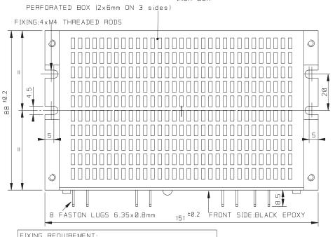
FIXING REQUIREMENT: The plate must be fix on a metallic surface. USE OF THERMIC GREASE IS NOT NECESSARY.
